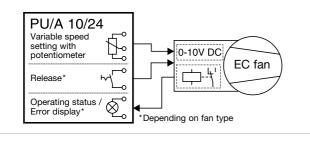
Speed potentiometer PU/PA with additional functions Switch and LED
