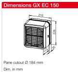
Low-noise window fans for use in private, commercial and industrial buildings. The series GX offers smooth running and functional reliability in continuous operation. The fan and external grille come in pleasant white. Attractive design, integrates unobtrusively in all rooms and any building facade.
