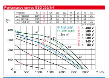
Performance curves GBD 355/4/4 T120 Frequency Hz 125 250 500 1k 2k 4k 8k L<sub>WA</sub> Radiation dB(A) 56 48 52 49 47 44 41 38 55 61 63 62 63 ∆p<sub>fa</sub> Pa Inlet side dB(A) 69 58 48 Lwa dB(A) 71 55 63 64 66 65 57 49 L<sub>WA</sub> Outlet side Centr. outlet 1 \( 400 V 400 - See left 2 A 280 V 69 3 Y 400 V ④ △ 200 V 68 300 5 △ 140 V 6 🛆 80 V 69 200 70 100 0 0 1000 2000 3000 ₿ m³/h
