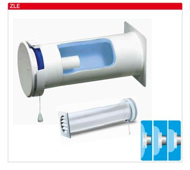
Special features – Application Manually operated supply air element for rooms of any kind. The volume flow is changed by a four-level locking mechanism. Adjustment by means of a freehanging drawcord. The supply air flows in through the disc valve optimally distributed, filtered (class G31) and sound-insulated.
