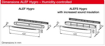
Humidity-controlled intake air elements ALEF Hygro with volume flow control/limitation, for installation in window frames/leaves.
