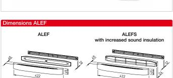
Intake air elements ALEF with volume flow control/limitation, for installation in window frames/leaves.
