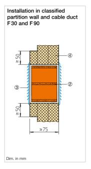
Fire protection ventilation tiles for the supply and extract ventilation of closed rooms and chambers to be protected against the spread of fire and smoke, such as e.g. installation shafts and cable ducts. They allow a constant, static air exchange which prevents heat accumulation in the closed chambers.
