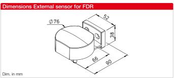
Differential humidity controller incl. integrated sensor for inside humidity and temperature, external sensor for intake air humidity and temperature as well as the necessary switching power supply.
