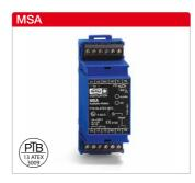
When a PTC thermistor reaches the nominal response temperature, the built-in relay drops out. Faults are indicated by the built-in LED. Recommissioning by pressing the "Reset" button or via external connectable switches. Plastic casing for switch cabinet installation on mounting rails according to DIN EN 60715.
