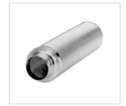
Flexible cross talk silencer FSD 200 Ref. no. 00679 Made of aluminium pipe with double-sided plug-in connectors. Sound insulation lining 50 mm thick, installation length 1 m.
