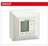
WSUP Ref. no. 09990 Digital timer with illuminated LCD display for automatic controlling the operating modes of any units up to 10 A rated current. Suitable for switching the smallest electric currents from 1mW (0.1V/1mA) through standard, gold-plated μ contact. 56 programmable switching times for all weekdays. With
