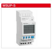
WSUP-S Ref. no. 09577 Digital timer with illuminated LCD display for automatic controlling the operating modes of any units up to 16 A rated current. Suitable for switching the smallest electric currents from 1mW (0.1V/1mA) through standard, gold-plated μ contact. 56 programmable switching times for all weekdays. With smartphone via NFC (free App).
