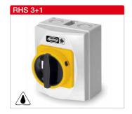
RHS 3+1 Ref. no. 01594 "0" position can be locked with a padlock. In accordance with DIN EN 60204 p.1/VDE 0113-1. Plastic casing for surface-mounted installation. 3-pole with auxiliary contact, for single-speed and speed-controlled fans.
