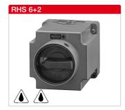
RHS 6+2 Ref. no. 01595 "0" position can be locked with a padlock. In accordance with DIN EN 60204 p.1/VDE 0113-1. Plastic casing for surface-mounted installation. 6-pole with 2 auxiliary contacts, for all pole-changing fans.
