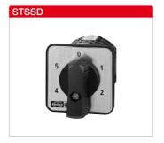
Five-step operating switch STSSD compatible with speed control transformer TSSD for 3~, 400 V fans. For switch cabinet installation with front attachment and front plate. Recessed connections.
