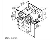
outside of casing; can be rotated into any position.
