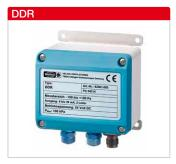
Duct smoke detector with VdS, incl. inlet duct for early detection of fire gases in the outside air inlet at flow speeds of 1 - 20 m/s. Operating current 16-28 V DC. Power consum. rest/alarm 22/11 mA. Protection class IP54. Relay contact potential-free break contact.
