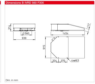
High-quality, high-performance jet fans with optimal dimensions for minimum space requirement. Suitable for supply and extract ventilation of car parks. Temperature range 300 °C/120 min. (in smoke extraction operation) or 60 °C in permanent operation.
