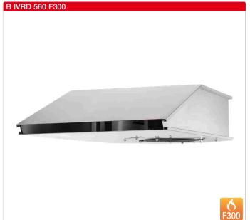
High-quality, high-performance jet fans with optimal dimensions for minimum space requirement. Suitable for supply and extract ventilation of car parks. Temperature range 300 °C/120 min. (in smoke extraction operation) or 60 °C in permanent operation.
