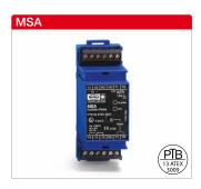
When the nominal response temperature of a PTC thermistor is reached, the built-in relay drops out. A fault is indicated by built-in LED. Recommissioning by pressing the "Reset" button or via externally connectable switch. Plastic casing for switch cabinet installation on mounting rail according to DIN EN 60715.
