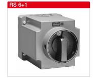
Voltage 400 V, 3~, 50/60 Hz. Protection category IP65. Protection class II. Actuation Rotary actuator. Locking options. "0 OFF" and "I ON". Temperature range -25 °C to +60 °C. Casing Flush and weather-resistant. Wiring diagram no. 1088
