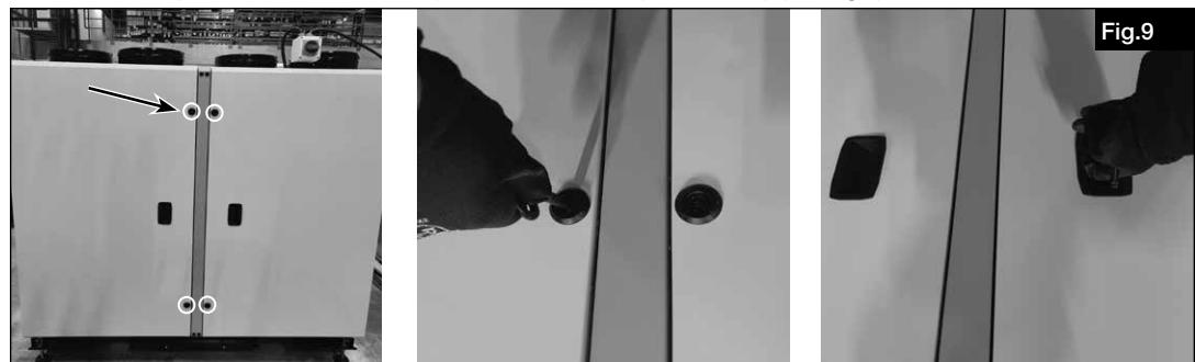
5. Remove the condensate cap with a screwdriver (see Fig.10).
