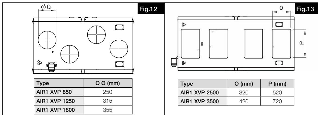
The dimensions for the unit flange connections can be found in the following table.
