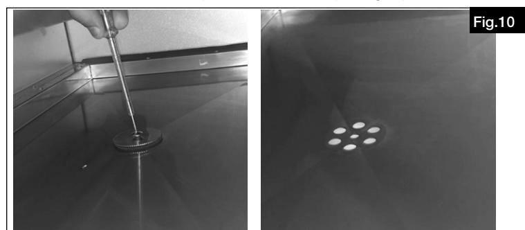
6. Unscrew the condensate cap from the screw and tighten the screw with a screwdriver (see Fig.11).
