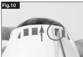
Fig. 10: Carefully pry up locking catch.
