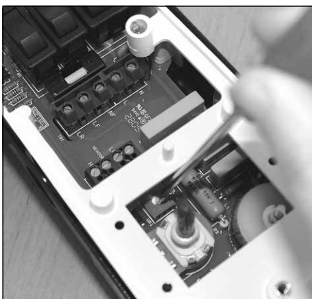
Fig. 2d: Potentiometer for setting the minimum speed
