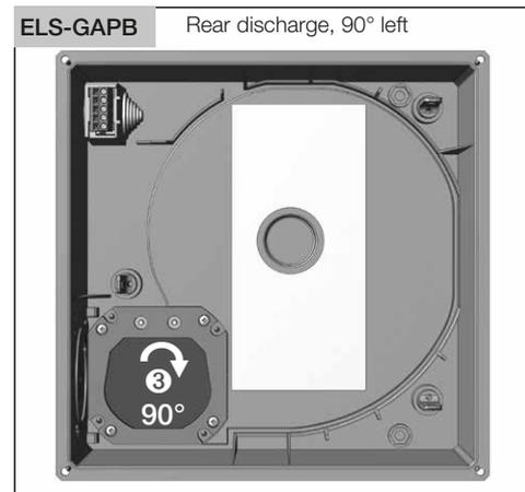
4.3 Install surface-mounted casing ELS-GAP
