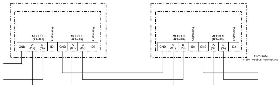
The connections for MODBUS “A (D+)”, “B (D-)” are available double and are connected with each other internally.
