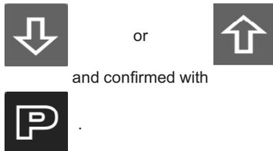
After setting the "language" and "mode" the desired "nominal value" is set, followed by the "control range". Select respectively with the "Up" and "Down" keys and confirm with "P".
