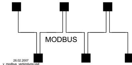
The data line must be conducted from one device to the next. No other type of wiring is allowed!
