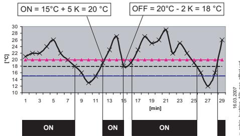
If the ambient temperature is higher than the set operating point, the cooling remains switched on. If the ambient temperature falls below the set operating point of the cooling by 2 K (Kelvin), it is switched off. I.e., the OFF point is situated at the hysteresis value under the ON point.
