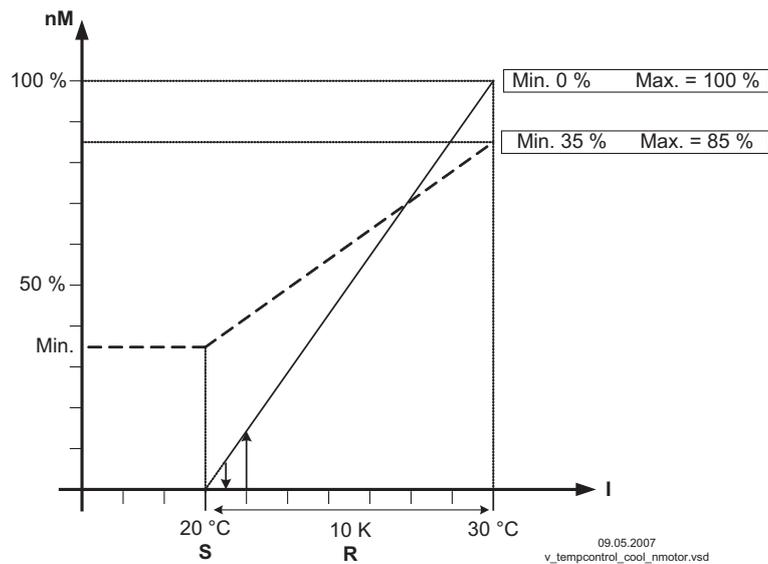
(Controller Setup: “Val > Set = n+” to “ON”)
