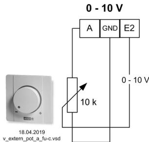
**External Setpoint** via external signal instead of "Setpoint 1". The "external Setpoint" function must be activated in base setup  $\overline{1E}$  for "E2 function". The active external Setpoint value is displayed in the "info" menu group.
