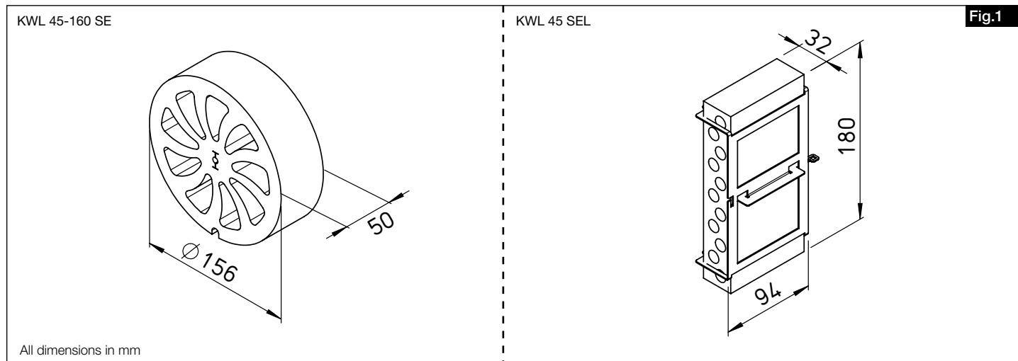
**Sound Insulation Element KWL 45-160 SE for wall installation sleeve
