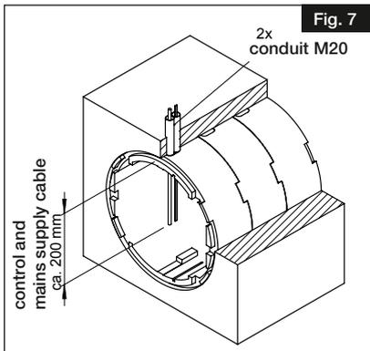
3.3 Installation of KWL EC 60 Pro fan unit
