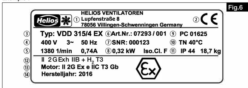
Zeichenschlüssel Typenschild Ventilator:
