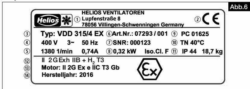
Zeichenschlüssel Typenschild Ventilator:
