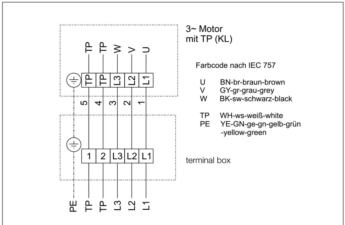
WIRING DIAGRAM OVER-
