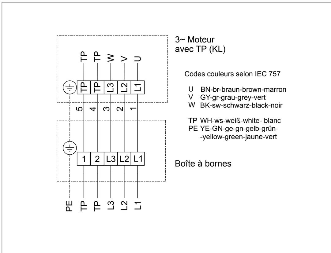
SCHÉMAS DE RACCORDEMENT RD/VD TYPES EX Ø 315-630
