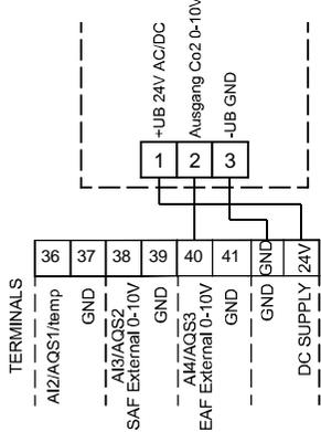
36-37: Air Quality Sensor 1 or temperature sensor (temp output AIR1/KWL-FTF 0-10V)
